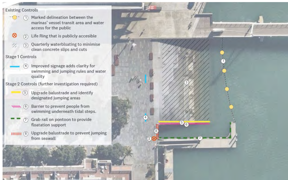
Figure 2: Karanga Plaza Tidal Steps Proposed Engineering for summer 2022-23
